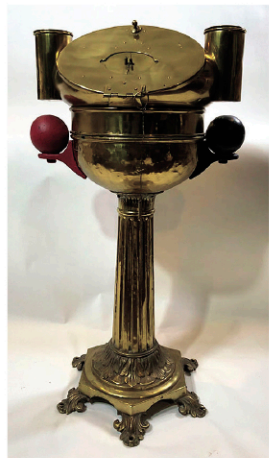
Rare nineteenth century solid brass yacht binnacle with gimballed compass marked with the maker's name Whyte Thomson Companies of 96 Hope St, Glasgow. Compass is polished and lacquered
