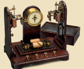
Bright’s Bell Acoustic Telegraph Sounder, 1855 The earliest form of acoustic telegraph instrument used in Great Britain. Estimate: 3.000–5.000€ / $ 3,300–5,500
